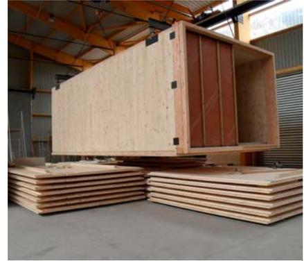
Prefabricated housing module made of CLT panels.
