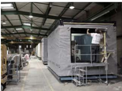
Prefabricated boxes Pictures of the manufacturing and assembly process
